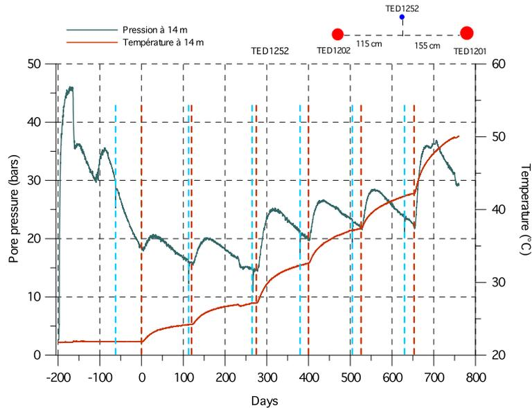
Figure 1 Pore pressure and temperature measurements in TED experiment. Dates of permeability tests are represented in blue dashed lines and dates of heating step in red dashed lines
